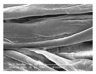
Figure 1: Scanning Electron Photomicrograph of Untreated Cotton Fabric at 20 µm
