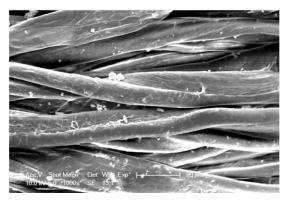
Figure 2: Scanning Electron Photomicrograph of Benzophenone-2 Treated Cotton Fabric at 20 µm
