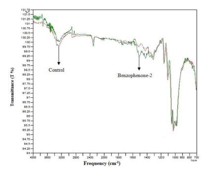
Figure 3: FTIR of Untreated and Benzophenone-2 Treated Cotton Fabric
